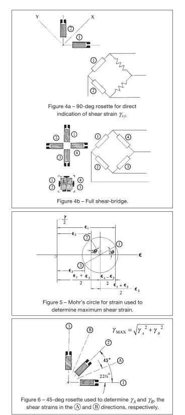
**Plane-Shear Measurement with Strain Gages**
