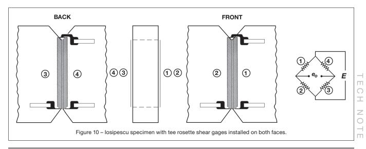
Plane-Shear Measurement with Strain Gages
